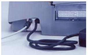
4. Plug the power cord into a power outlet.
